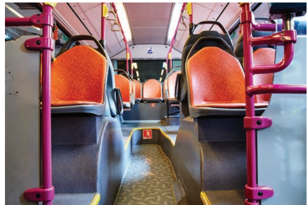
Newer barrier-free bus design with slope, but which still require a step up for commuters to sit at the back half of the bus
